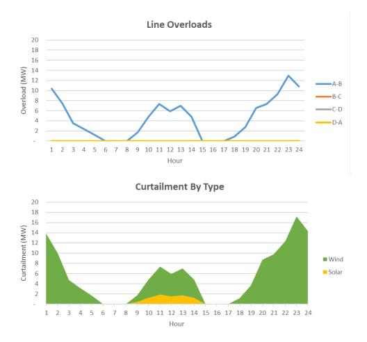
Note that, for this example system, if only one of the technology types is producing energy at the time of line overloads, the amount of curtailment necessary to remedy line overloads will exceed the overload amount. This is due to a particular generators shift factor relationship to the overloaded line.
