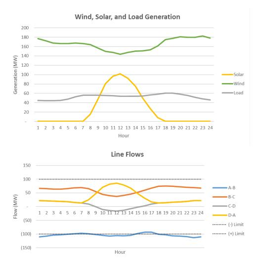
The charts show the interaction between the varying dispatch patterns of the generators on the system with the transmission system. For the "A-B" transmission line, it can be noted that the
